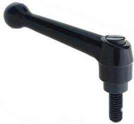
The locking levers allow easy positioning, tightening and holding adjustments. Simply lift the adjustable handle away from its threaded center to rotate freely. Then release the handle to engage and tighten. The handle of the locking lever can thus be rotated for easy tighten / release operations. Locking levers and more are available at [BeaumontMetalWorks.com](http://BeaumontMetalWorks.com)
